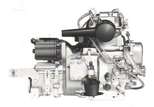
The BMW D7 Marine Engine: 4.5 kW (6 bhp). Particularly suitable for sailing boats and open displacement boats up to approx 7.5 metres (24') and 2 tons.
