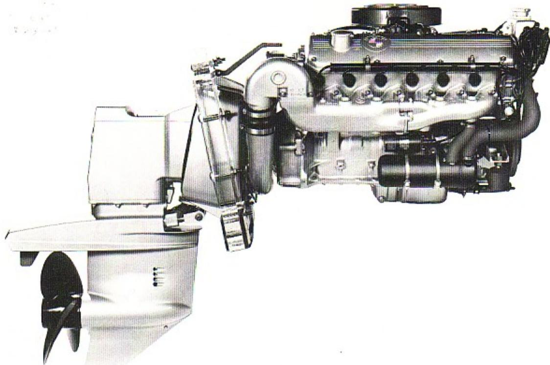
**The BMW B190 Z Marine Engine with stern drive: 121 kW (165 bhp). Particularly suitable for fast planing cruisers up to 2 tons. In both single and twin installations.**
